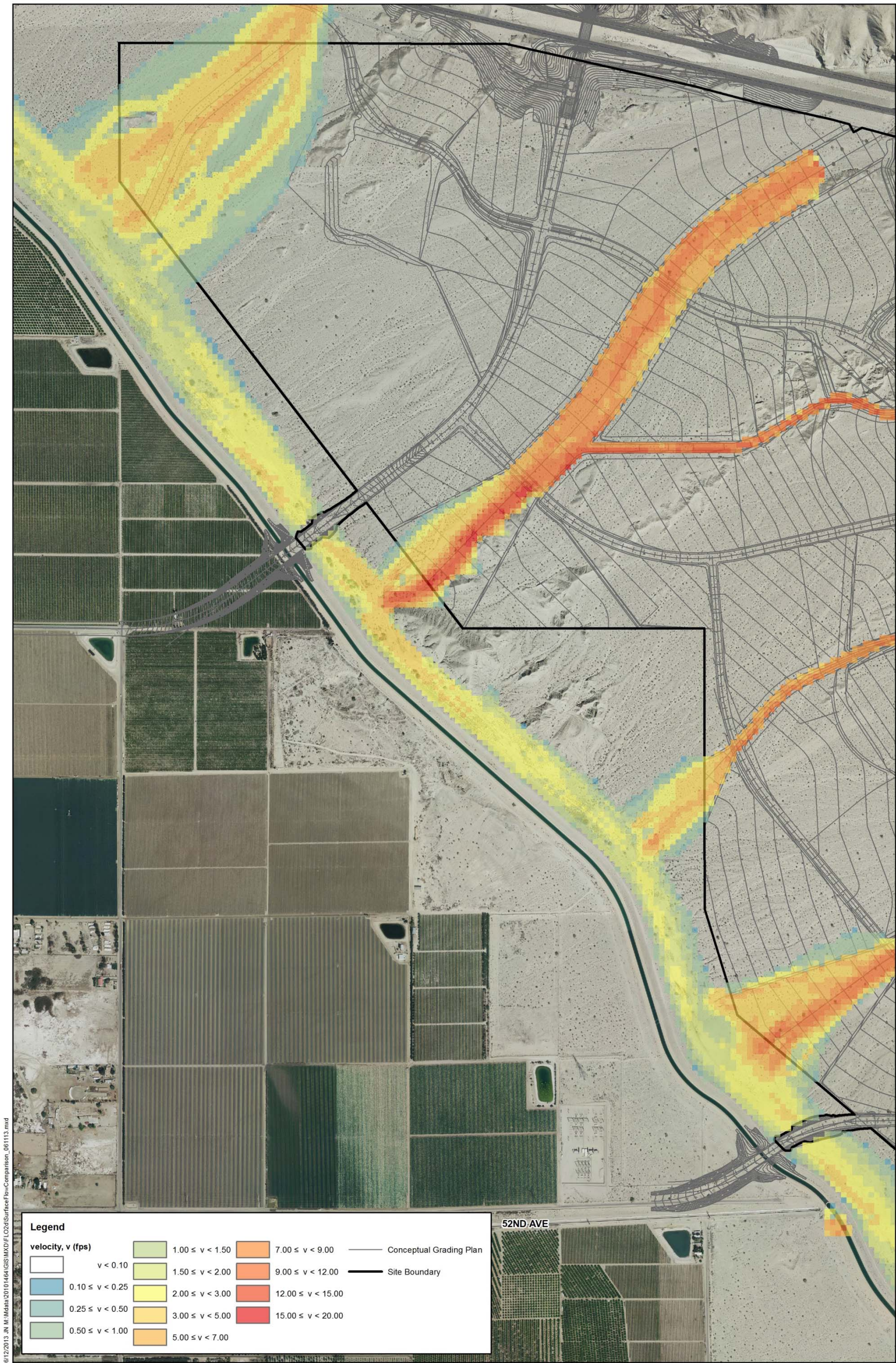
Figure 3-35. Project with crossings SPF maximum flow velocities
